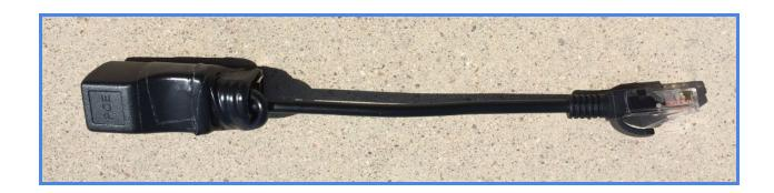
This mod works on either the male or female adapter, so you can make two of these per set of PoE adapters. The power lead is trimmed so it can be soldered to the + and - points on the circuit board. Wrap in Kapton tape and secure with heat shrink. Weather-proof the adapter as needed, or secure it in an enclosure with the device being powered.
