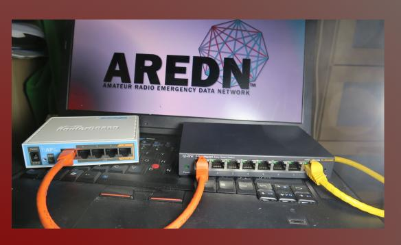
Connect an Ethernet cable from your computer to the switch, and another from the LAN port of the PoE adapter to the switch.
